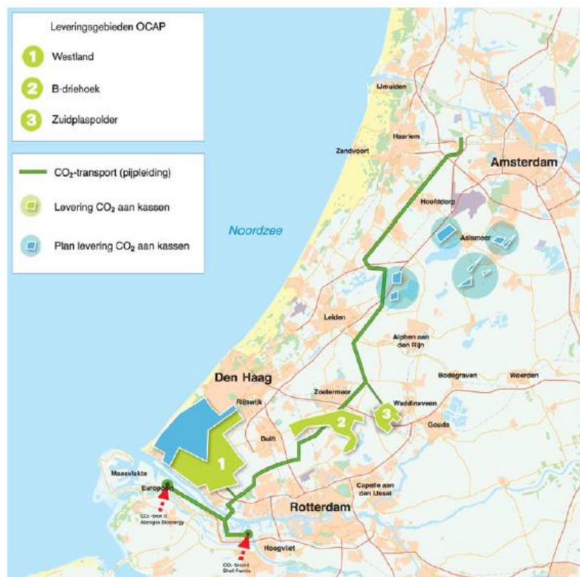
Figure 2: The OCAP pipeline, CO 2 sources (red arrows) with current (green) and planned (blue) CO 2 delivery areas
