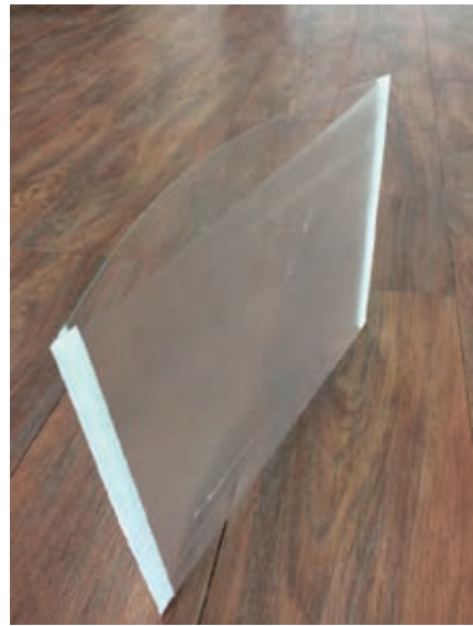
Figure 10 Insulating roof with cold bended thin glass (Leoflex™ or Falcon™) on top and flat ETFE foil (F-Clean ® ) below.
