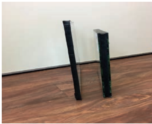
Difference between double insulating glass made from 2x thin glass (left) and 2x4 mm glass (right)
