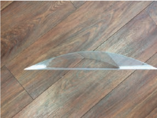
Figure 11 Insulating roof with cold bended thin glass (Leoflex™ or Falcon™) on top and flat glass below, or vice versa.
